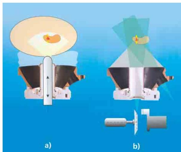
Fig. 8: a) Inline Ultrasound b) Inline X-ray
